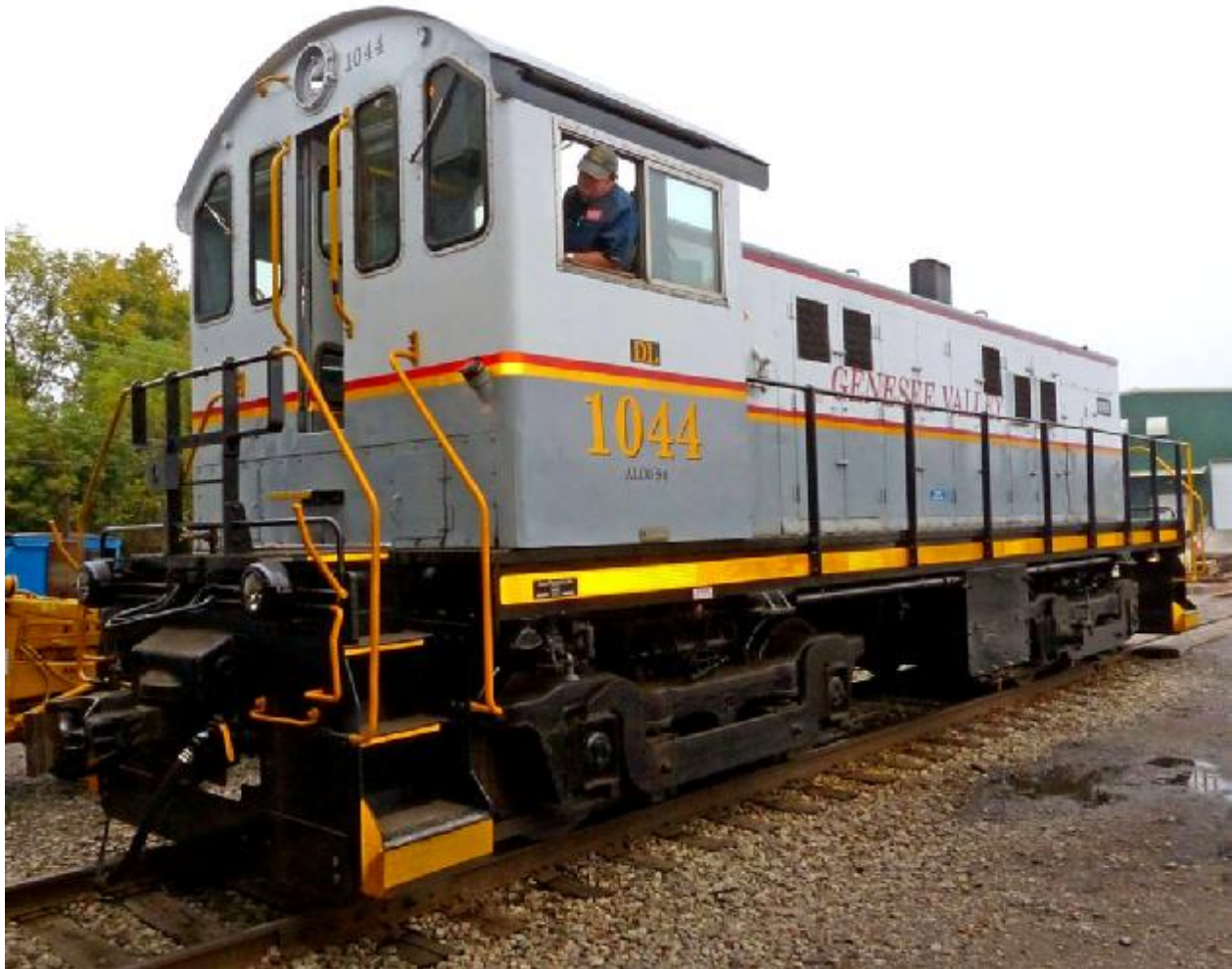
Neil Keirn at the helm of the Genesee Valley Transportation # 1044 Alco S6 diesel.
